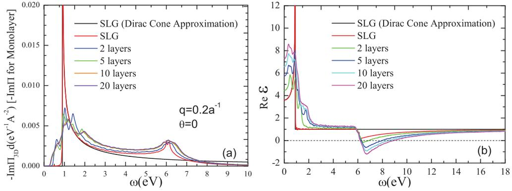
FIG. 11. (Color online) (a)  $\text{Im}\Pi(\mathbf{q}, \omega)$  for SLG and MLG. The results for SLG obtained from the Kubo formula Eq. (4) are compared to those obtained from the Lindhard function Eq. (11), and to the Dirac cone approximation. (b)  $\text{Re}\epsilon(\mathbf{q}, \omega)$  for SLG and MLG and comparison to the Dirac cone approximation, for the same value of  $q$  as in (a).
