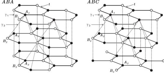
FIG. 1. Atomic structure of ABA- and ABC-stacked multilayer graphene. The intralayer ( $t$ ) and interlayer ( $\gamma_1$  and  $\gamma_3$ ) hopping amplitudes are considered, as explained in the text.
