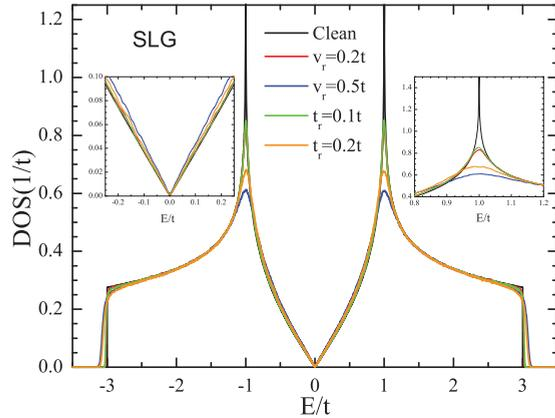
FIG. 4. (Color online) Density of states for SLG considering different kind of disorder. The left inset shows a zoom of the DOS near the Dirac point ( $E = 0$ ), whereas the right-hand side inset shows the disorder broadening of the Van Hove singularity at  $E = t$ . The numerical method used in the calculation of DOS is described in Ref. 29, and the sample size of SLG is  $4096 \times 4096$ .
