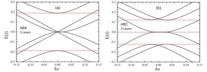
FIG. 9. (Color online) Band structure of ABA- and ABC-stacked trilayer graphene. Left panel: The red dashed lines indicate the position of the jump in DOS of ABA-stacked trilayer graphene at  $|E| \approx 0.19t$ . Right panel: The red dashed lines indicate position of the peaks in DOS of ABC-stacked trilayer graphene at  $E = 0$  and  $|E| \approx 0.12t$ .
