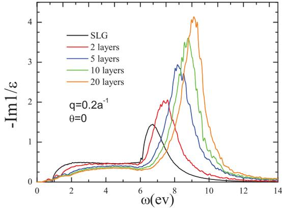
FIG. 13. (Color online) Loss function  $-\text{Im}1/\varepsilon(\mathbf{q}, \omega)$  for SLG and MLG, which is proportional to the spectrum obtained by EEL experiments (Ref. 3). We have used the same  $q$  as in Fig. 11.
