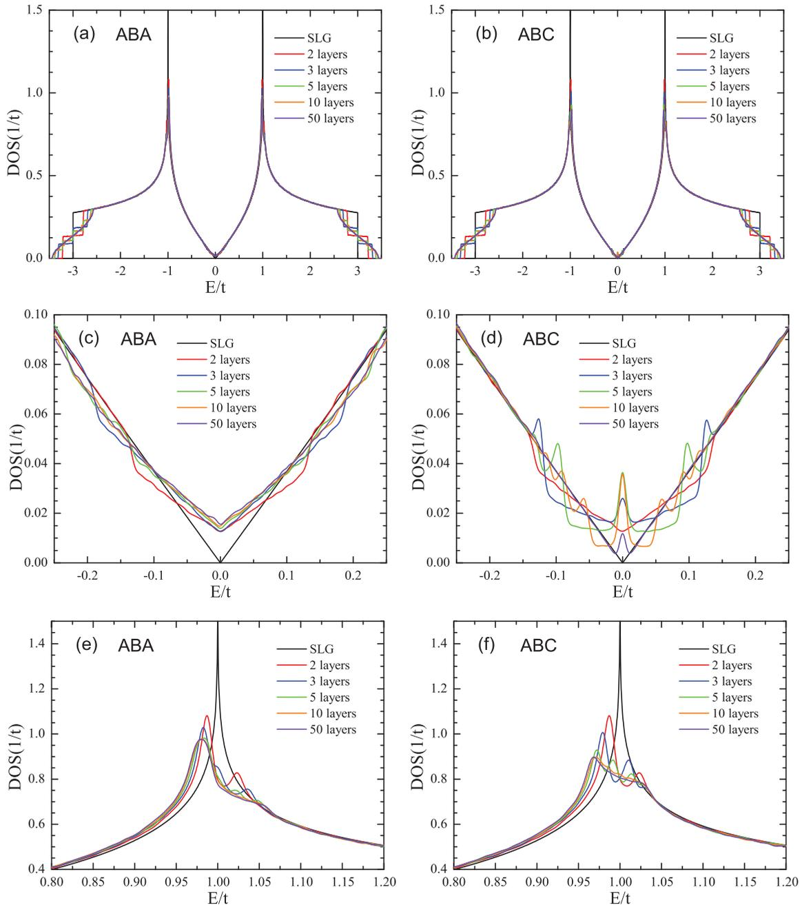
FIG. 8. (Color online) (a,b) Density of states of ABA- (left panels) and ABC-stacked (right panels) multilayer graphene. A zoom of the DOS around the Dirac point ( $E = 0$ ) is shown in (c,d), and around the Van Hove singularity ( $E = t$ ) is shown in (e,f). The sample sizes of each layer in MLG are  $4096 \times 4096$  atoms in bilayer;  $3200 \times 3200$  in trilayer;  $2048 \times 2048$  in five layers;  $1600 \times 1600$  in ten layers and  $800 \times 800$  in 50 layers.
