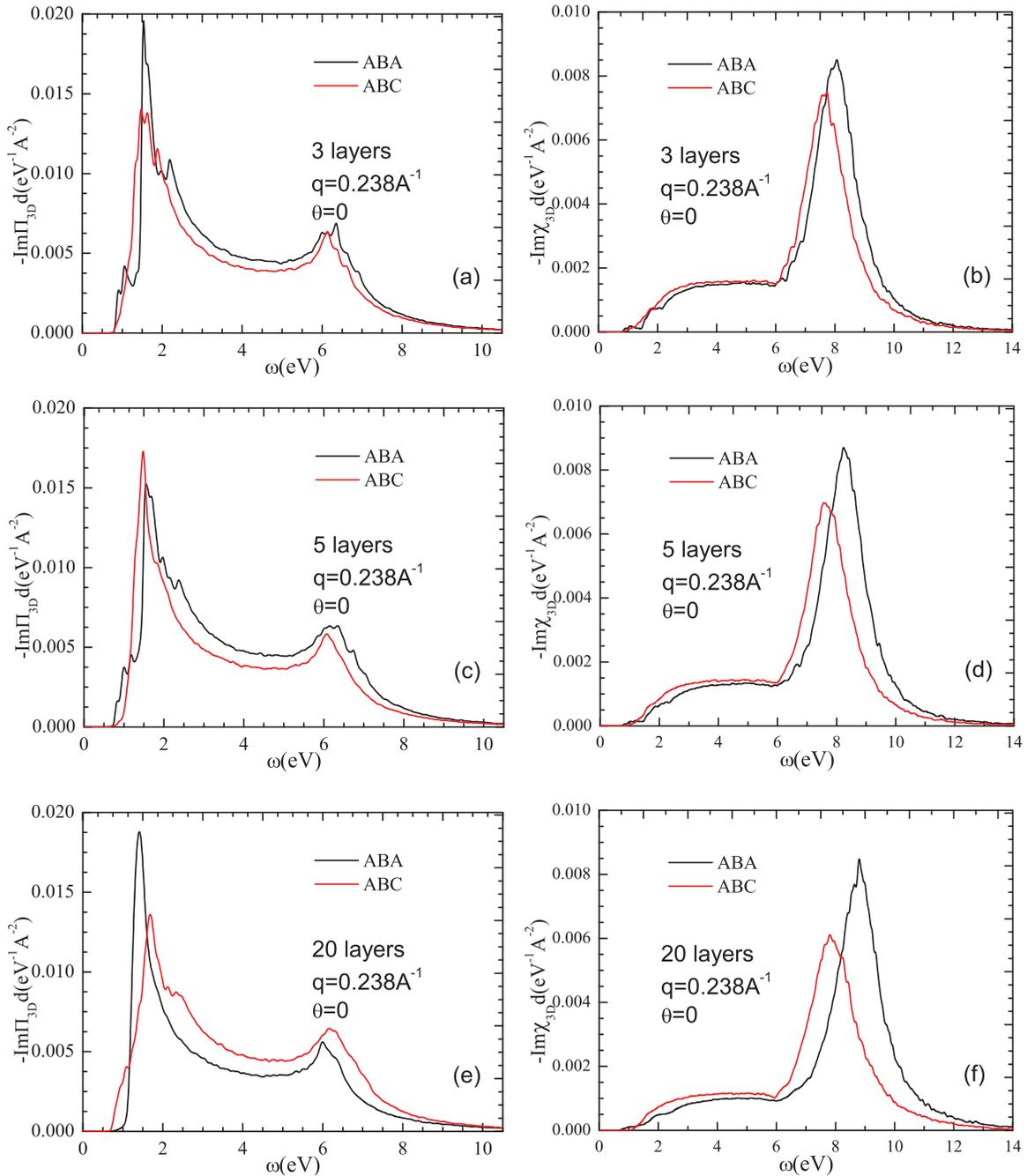
FIG. 10. (Color online) Dynamical polarization and response function of ABA- and ABC-stacked multilayer graphene. The number of layers are three layers in (a,b), five layers in (c,d) and 20 layers in (e,f). The size of each layer is  $3600 \times 3600$  atoms for trilayer (a,b);  $3200 \times 3200$  atoms for five-layer samples (c,d), and  $1600 \times 1600$  atoms for 20 layer (e,f).
